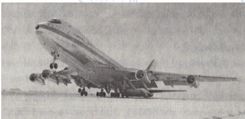
V_{mu} certification test
