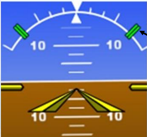
Nominal roll attitude ESP engagement limit indications
