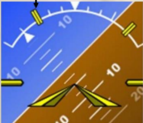
Engagement limit indications upon ESP activation
