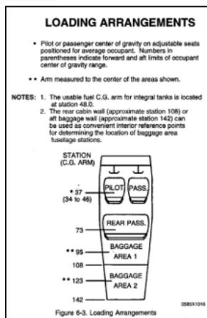
37 inches x 25.4 = 940mm. Write this on the table. The aircraft BEW arm is found on the load sheet, write this on the table also.
